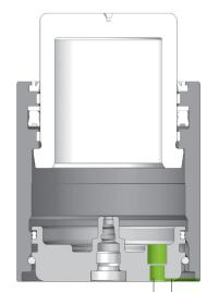
Rupture septum Exhaust groove
